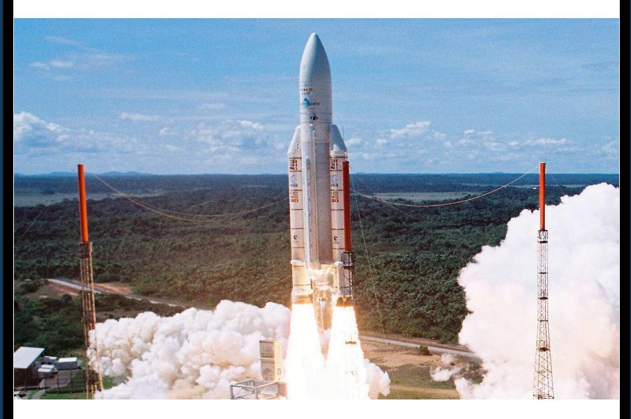
The Ariane 5 **reused** the code from the inertial reference platform from the Ariane 4, but the early part of the Ariane 5's flight path differed from the Ariane 4 in having higher horizontal velocity values. This caused an internal value BH (Horizontal Bias) calculated in the alignment function to be unexpectedly high.
