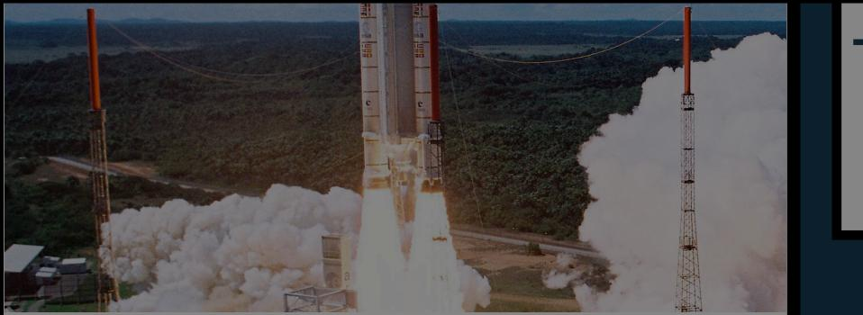
The Ariane 5 **reused** the code from the inertial reference platform from the Ariane 4, but the early part of the Ariane 5's flight path differed from the Ariane 4 in having higher horizontal velocity values. This caused an internal value BH (Horizontal Bias) calculated in the alignment function to be unexpectedly high.
